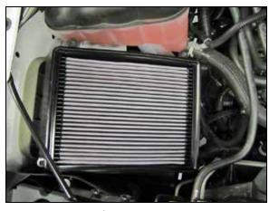
5. Install the AIRAID® air filter into the lower filter housing and then reinstall the upper housing and secure with the factory hardware.
