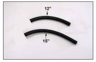
9. Cut the provided crank case vent hose into lengths of 12" and 15".
